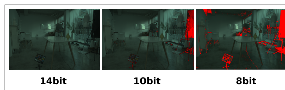
Fig. 4. Illustration of the increase of image noises due to the lower image bit-depth, with the noises shown in red. (Note: the noise was the difference between the 14-bit image and the images having lower bit-depths.)
